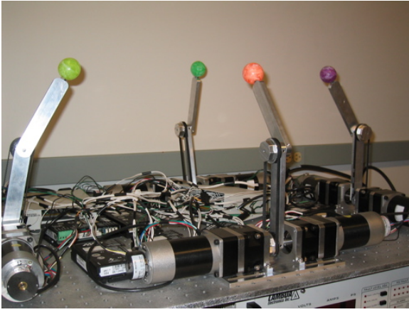
Fig. 1. An 8 degree-of-freedom four “finger” manipulator that manipulates objects it supports. The fingers are constrained, so stick/slip transitions between the actuator end-effectors and the manipulated object must occur when the actuators move.
