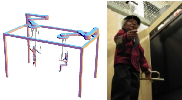
Fig. 1. A model of a robotic marionette stand and a photograph of the experimental marionette stand under development.
