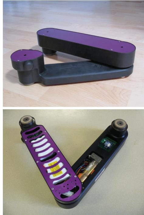
Fig. 2: (Top) Perspective view of the Gibbot. (Bottom) A view of the underside of the Gibbot.
