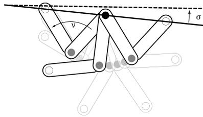
Fig. 6: An example of passive stable downhill brachiation on a slope of  $\sigma = 0.1$  radians and an interleg angle of  $\nu = 1.287$  radians.
