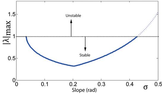
Fig. 8: The magnitude of the largest eigenvalue of the return map  $S$  of family C fixed points, plotted as a function of slope.
