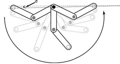
Fig. 10: An example of an actuated uphill brachiation on a slope of 0.024 radians.
