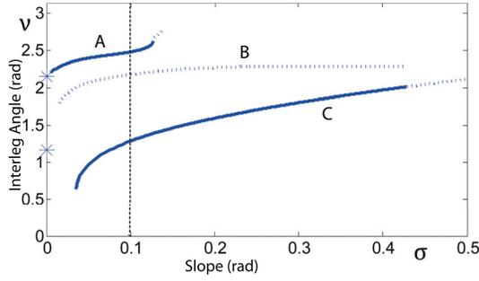
Fig. 7: Fixed-point families A, B, and C projected to  $(\sigma, \nu)$ . Solid lines indicate stable fixed points and dashed lines indicate unstable. Asterisks at zero slope indicate GR solutions. The dotted vertical line at a slope of 0.1 radians indicates the slice shown in Figure 9.
