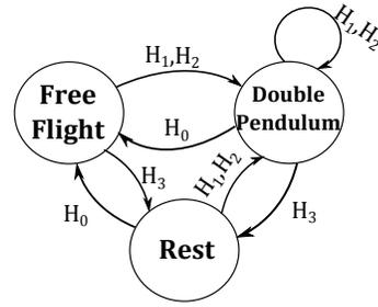
Fig. 4: The hybrid dynamics as a finite state machine.
