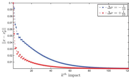
Fig. 11: The normed error between the uphill fixed point and the post-impact state due to small perturbations of  $\pm \frac{1}{10}$  radian to the interleg angle  $\nu$  at  $t = 0$ .
